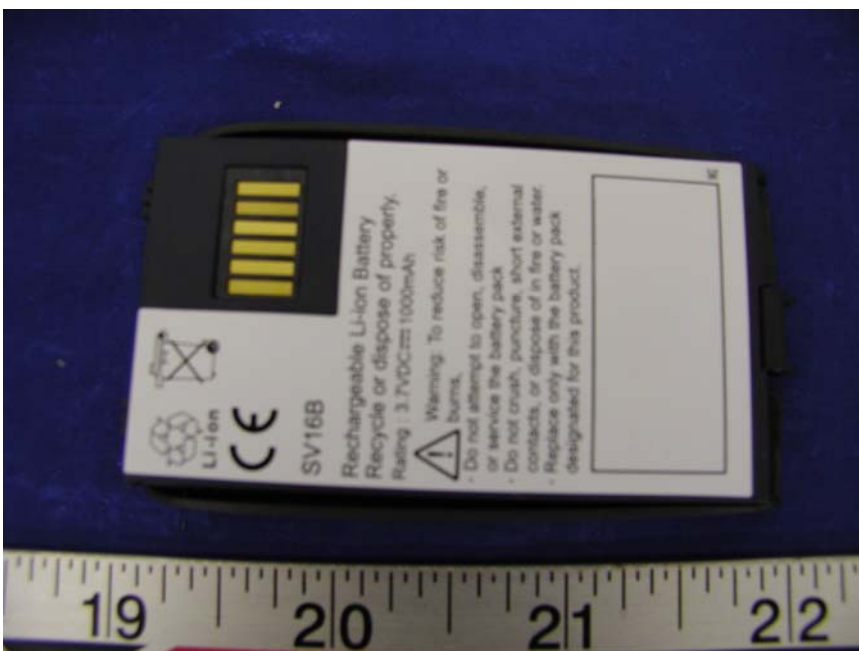
EUT – SV16B Dynapack Battery Rear View
