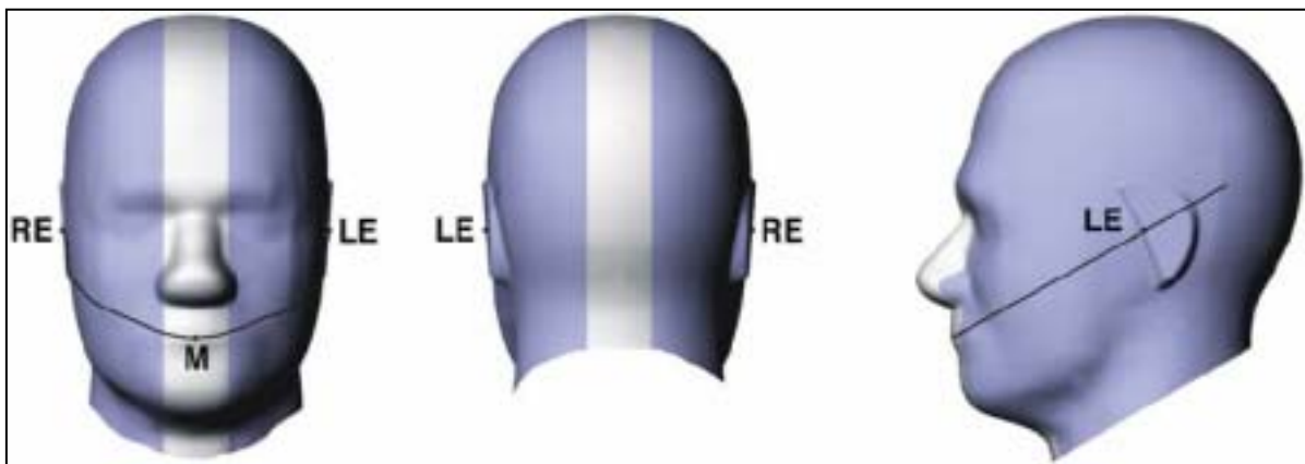
Figure 7-1a Front, back and side view of SAM (model for the phantom shell)
