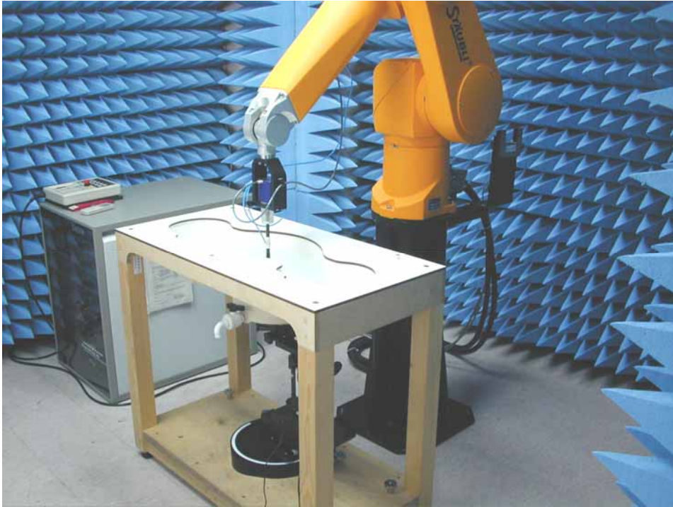
Fig.1 Photograph of the SAR measurement System
