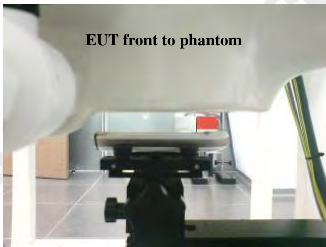
Fig.7 Body worn- EUT front to flat phantom and distance between flat phantom and mobile phone is 1.5 cm
