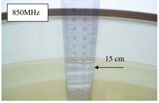
Fig.2.4 Photograph of the Tissue Simulant Fluid liquid depth 15cm for Flat (Body)
