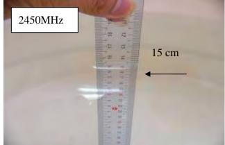
Fig.2.7 Photograph of the Tissue Simulant Fluid liquid depth 15cm for Flat (Body)
