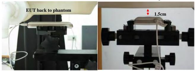
Fig.12 Body worn- EUT back to flat phantom and distance between flat phantom and mobile phone is 1.5 cm
