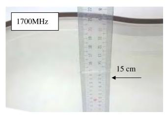
Fig.2.3 Photograph of the Tissue Simulant Fluid liquid depth 15cm for Right-head Side
