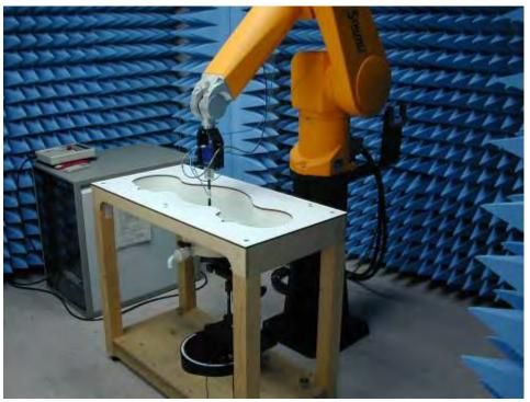
Fig.1 Photograph of the SAR measurement System
