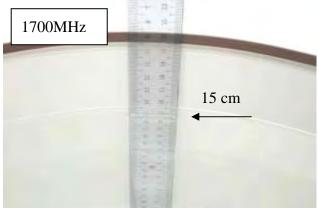
Fig.2.6 Photograph of the Tissue Simulant Fluid liquid depth 15cm for Flat (Body)
