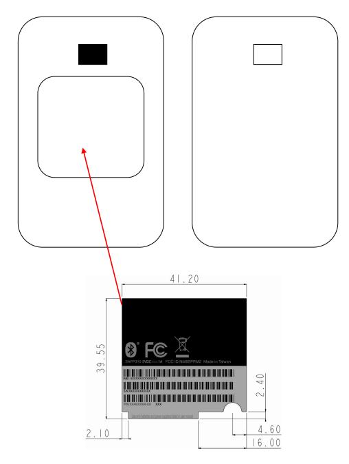
NOTE: label on internal PCB board, not on back cover
