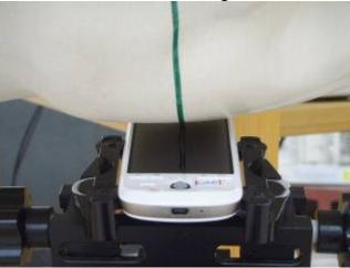
Fig.6 Left Head Section / Ear-Tilt Position(15°)
