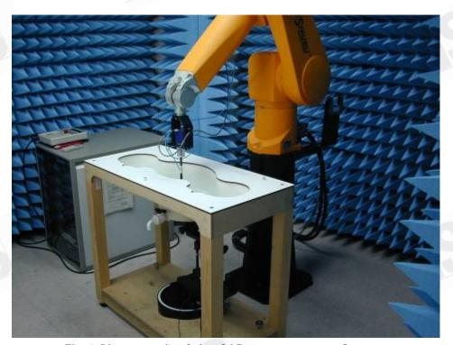
Fig.1 Photograph of the SAR measurement System
