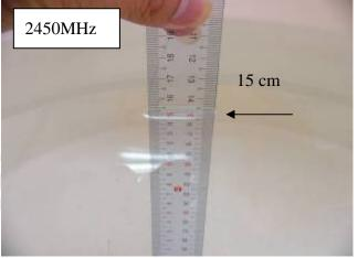
Fig. 2.7 Photograph of the Tissue Simulant Fluid liquid depth 15cm for Flat (Body)
