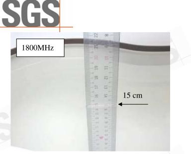
Fig.2.3 Photograph of the Tissue Simulant Fluid liquid depth 15cm for Right-head Side
