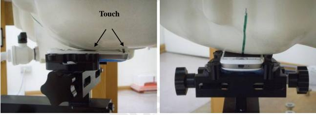
Fig.5 Left Head Section / Cheek-Touch Position
