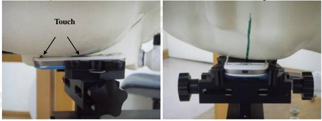
Fig.3 Right Head Section / Cheek-Touch Position
