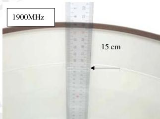
Fig.2.5 Photograph of the Tissue Simulant
