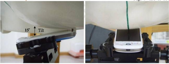
Fig.6 Left Head Section / Ear-Tilt Position(15°)
