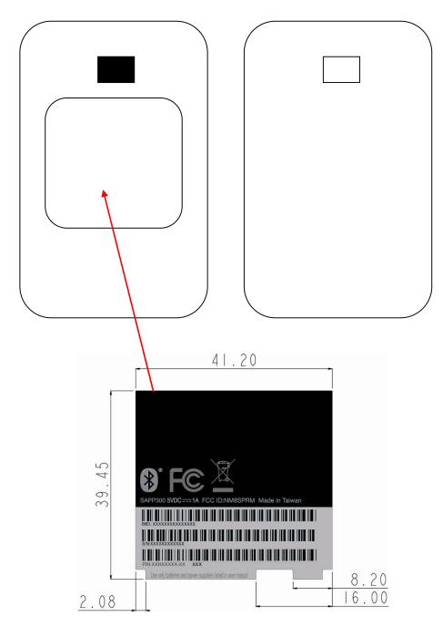
NOTE: label on internal PCB board, not on back cover
