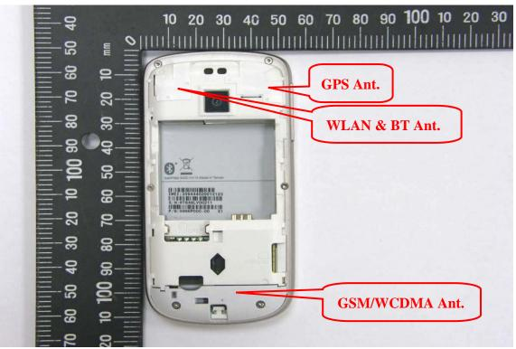
The min. distance is 8cm from GSM/WCDMA Antenna to WLAN/BT Antenna,
