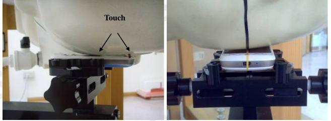
Fig.5 Left Head Section / Cheek-Touch Position
