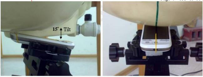
Fig.4 Right Head Section / Ear-Tilt Position(15°)
