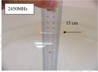
Fig.2.6 Photograph of the Tissue Simulant Fluid liquid depth 15cm for Flat (Body) Fig.2.5 Photograph of the Tissue Simulant Fluid liquid depth 15cm for Flat (Body)
