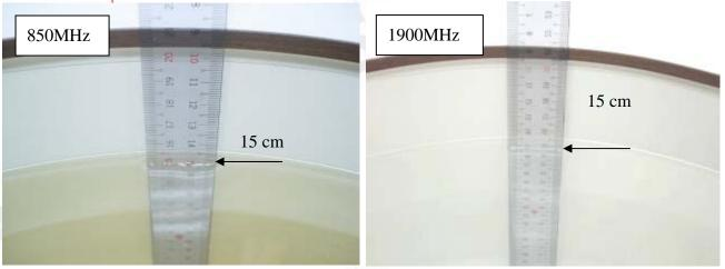
Fig.2.4 Photograph of the Tissue Simulant Fluid liquid depth 15cm for Flat (Body)
