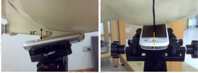
Fig.6 Left Head Section / Ear-Tilt Position(15°)
