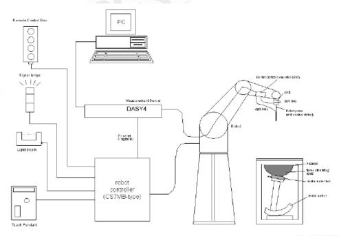
Fig.a The block diagram of SAR system
