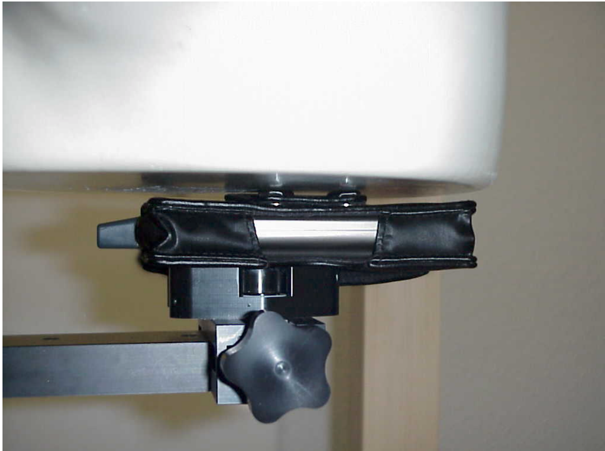
Photo 2: Position flat phantom, front side (body SAR measurement)
