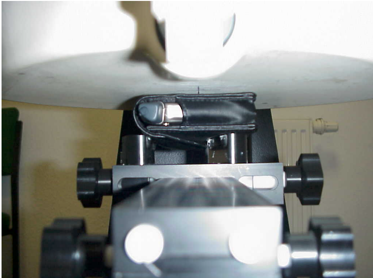
Photo 3: Position flat phantom, front side (body SAR measurement)
