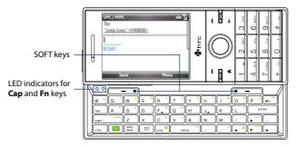
The LED indicators corresponding to the **Cap** and **Fn** keys on the keyboard display solid orange color when the and summer when the responding keys are pressed to turn on their functionality. Press a desired corresponding key and turn them off after use. You can do the following with the QWERTY keyboard:
