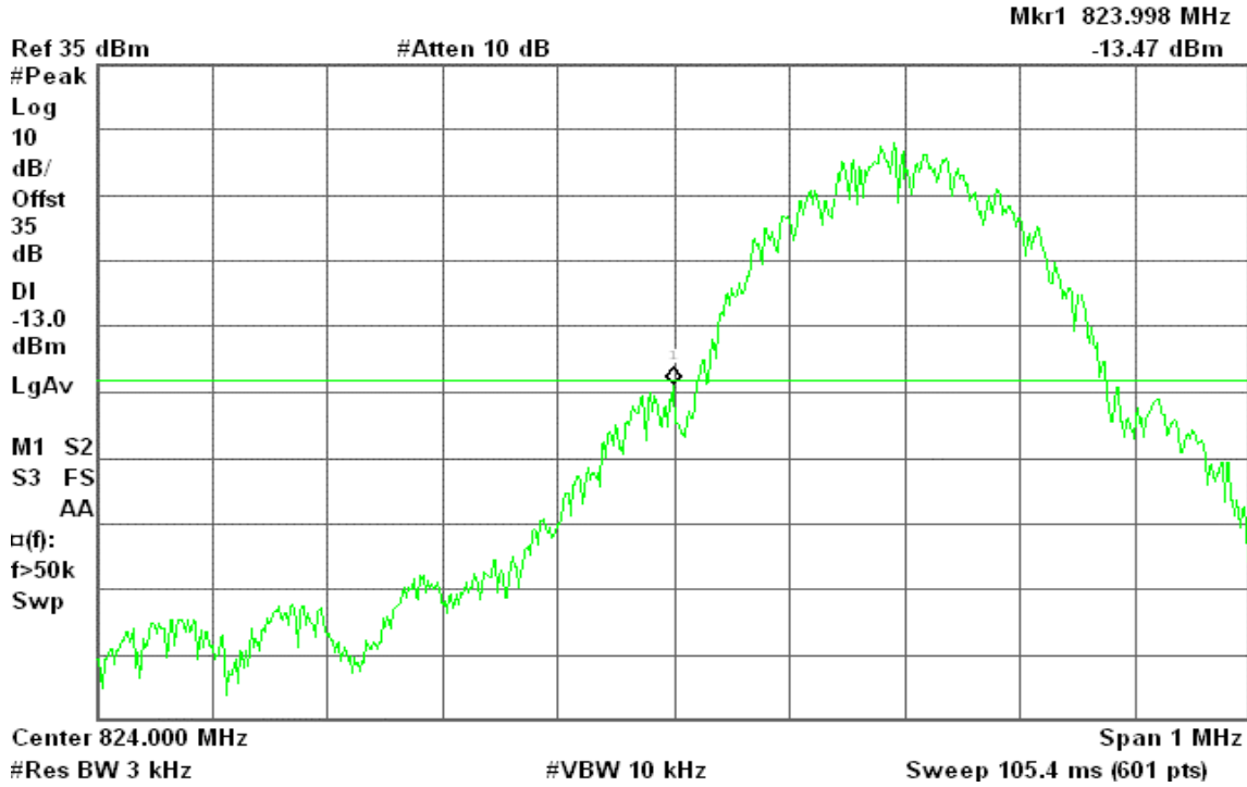
Figure 9-4: Band Edge emissions –GPRS CH High
