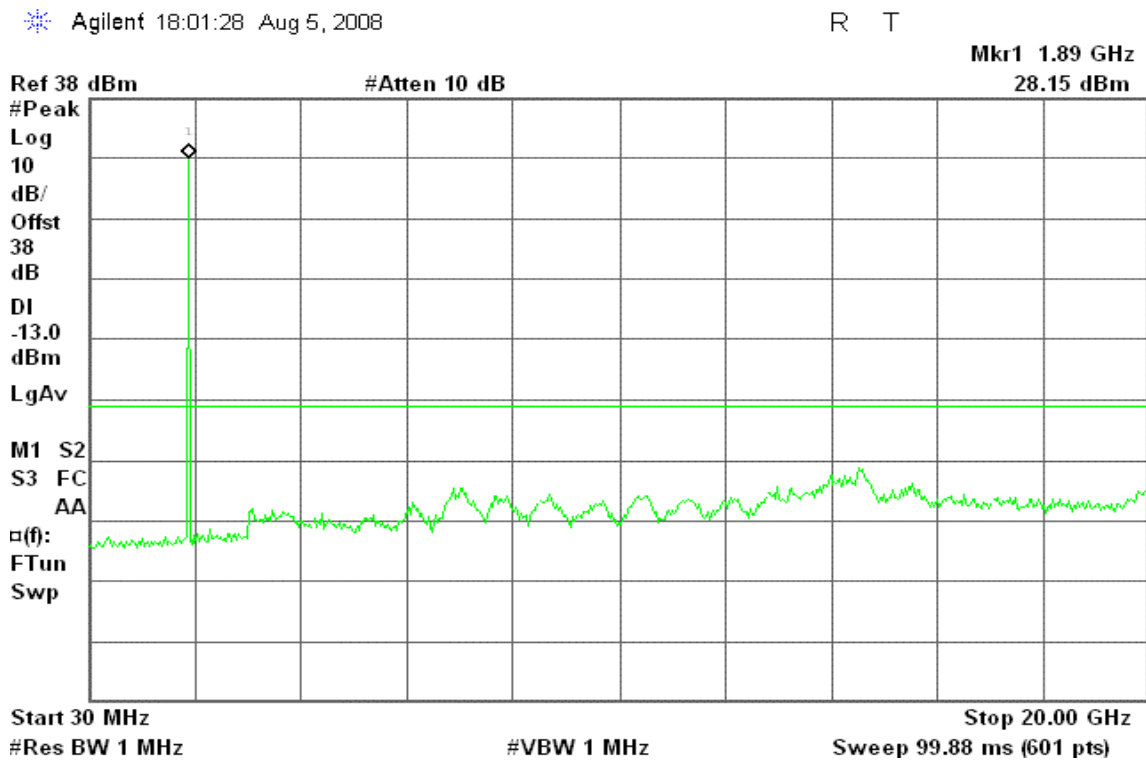
Figure 8-6: Out of Band emission at antenna terminals – GPRS CH High
