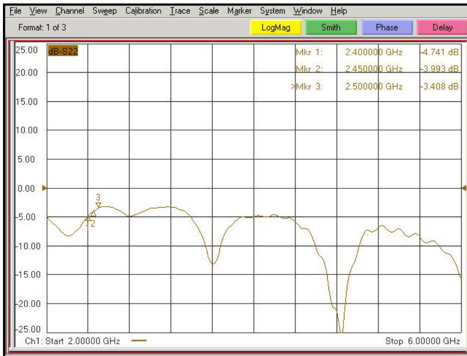
Figure 2. Return loss plot for the Bluetooth antenna in the IPAQX without any cards inserted.
