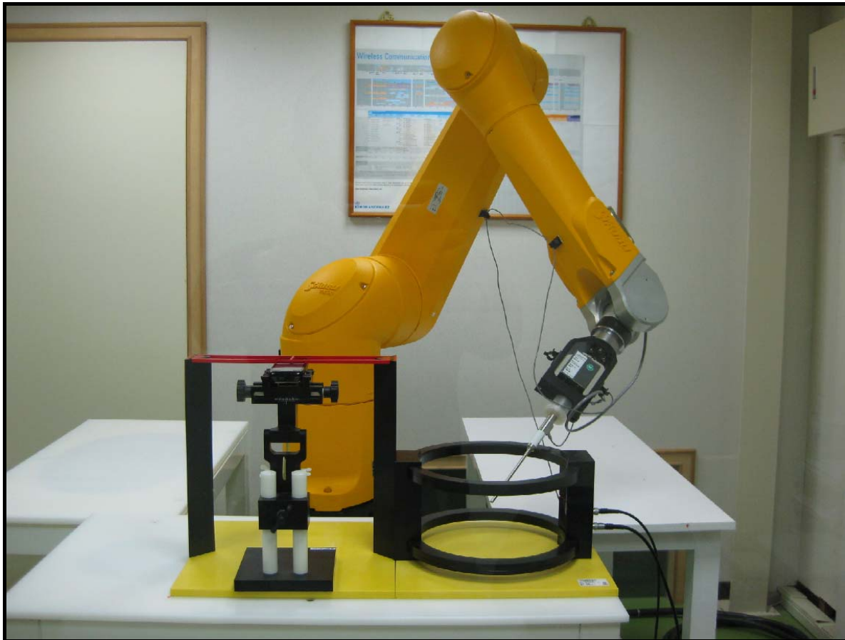
Figure 4.2: T-Coil setup with HAC Test Arch and AMCC
