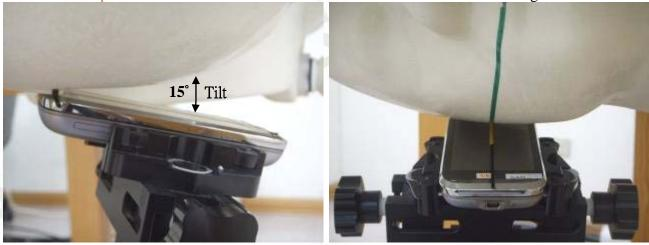
Fig.4 Right Head Section(Slider off)/ Ear-Tilt Position(15°)
