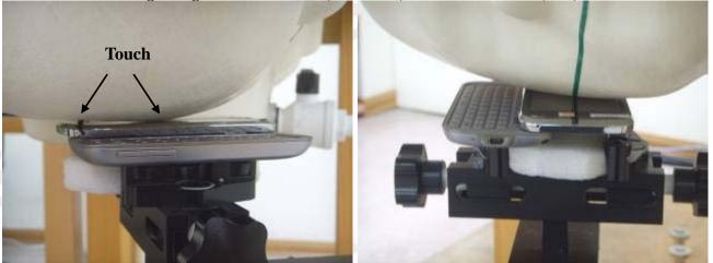
Fig.5 Right Head Section(Slider on) / Cheek-Touch Position
