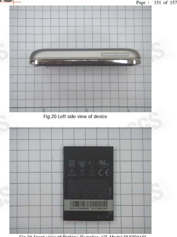
Fig.21 Front view of Battery (Supplier: HT, Model:RHOD160)
