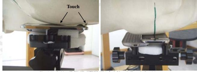
Fig.9 Left Head Section(Slider on) / Cheek-Touch Position
