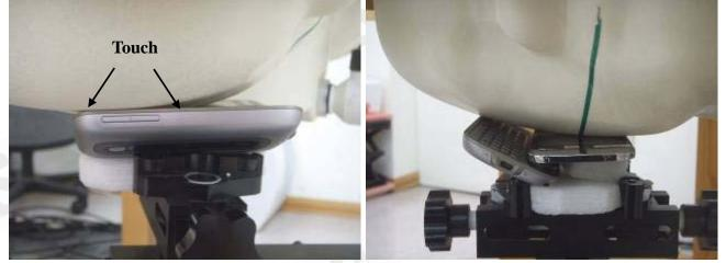
Fig.11 Right Head Section(Hold up) / Cheek-Touch Position
