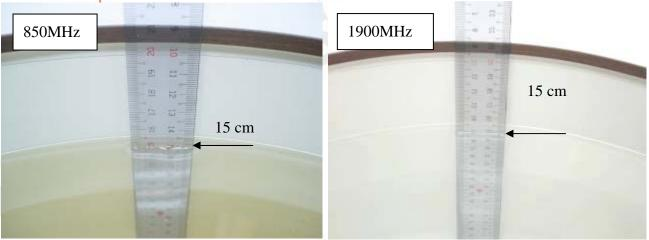
Fig.2.3 Photograph of the Tissue Simulant Fluid liquid depth 15cm for Flat (Body)
