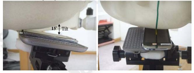
Fig.6 Right Head Section(Slider on)/ Ear-Tilt Position(15°)
