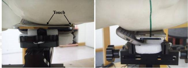
Fig.12 Left Head Section(Hold up) / Cheek-Touch Position
