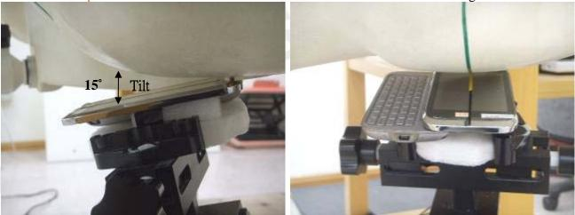
Fig.10 Left Head Section(Slider on) / Ear-Tilt Position(15°)
