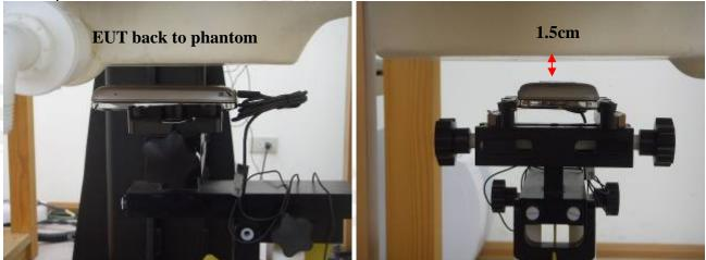
Fig.15 Body worn- EUT back to flat phantom and distance between flat phantom and mobile phone is 1.5 cm\_ repeated with headset
