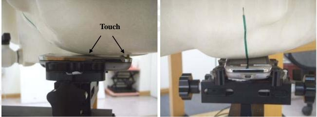
Fig.7 Left Head Section(Slider off) / Cheek-Touch Position
