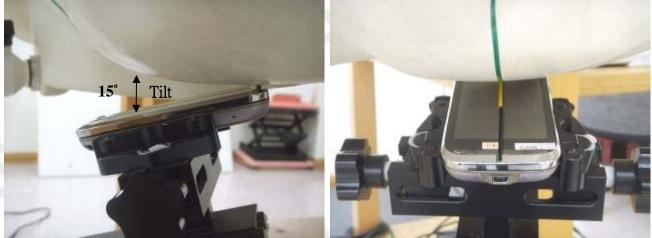
Fig.8 Left Head Section(Slider off) / Ear-Tilt Position(15°)
