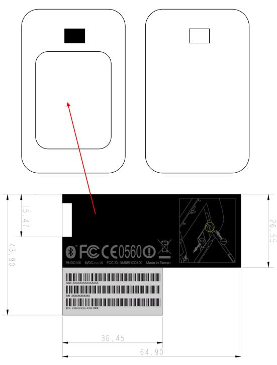
NOTE: label on internal PCB board, not on back cover
