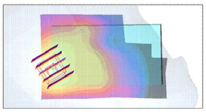
Response: The WiMAX antenna is located in the left top. Therefroe, hot spot is positioned in upper area scan and the vacancy of has no SAR spread, Also, it would not affect SAR evaluation.
