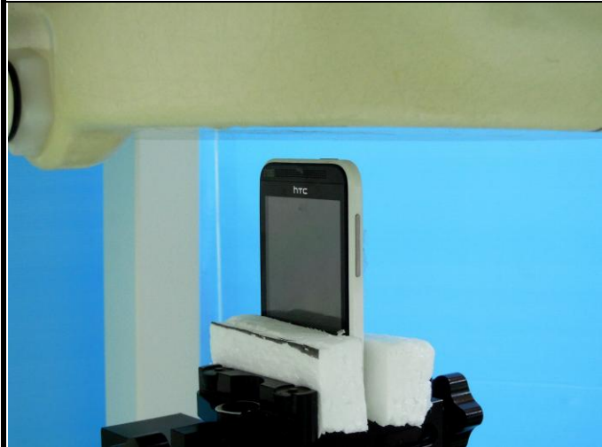
Top Side of EUT with 1.0 cm Gap
