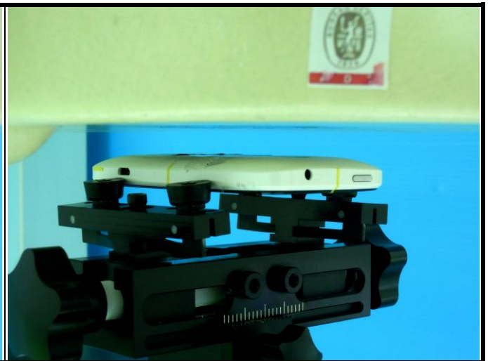
Rear Face of EUT with 1.0 cm Gap
