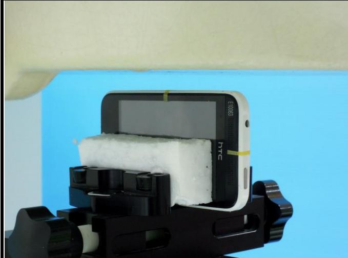
Left Side of EUT with 1.0 cm Gap
