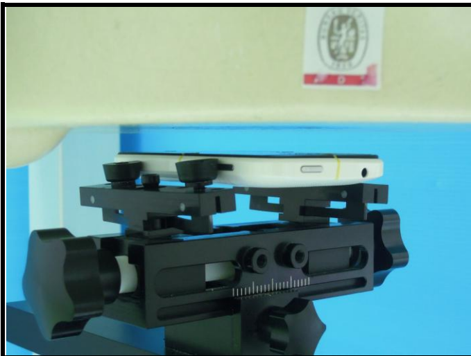
Front Face of EUT with 1.0 cm Gap
