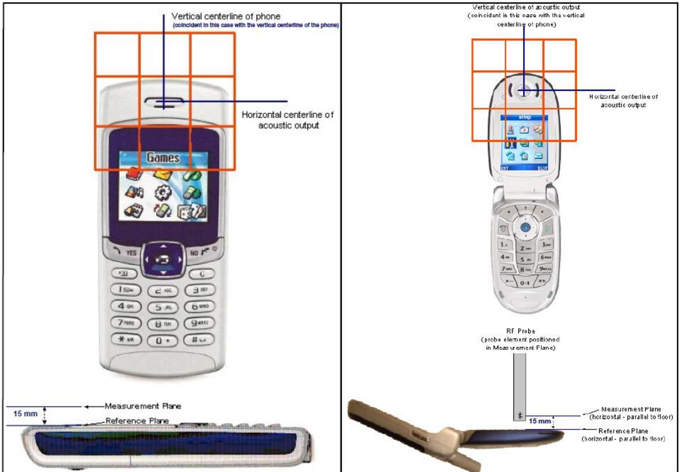
Fig-3.4 EUT Reference and Plane
