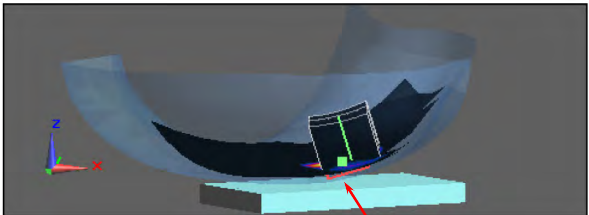
Figure 1. Right Head SAR Test Setup (Cheek)
