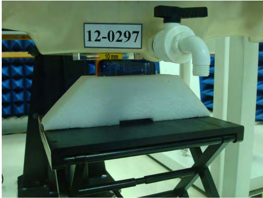
Figure 11. Body SAR Test Setup (Flat Section)
