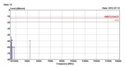
Site : 966 Chamber 5 Condition : PART22/24/27 3m EIRP\_RSE\_1G~19G\_3 HORIZONTAL
