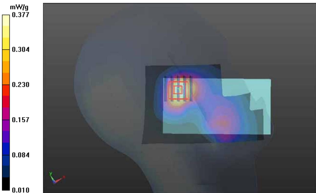
**P584 LTE 4\_QPSK\_10M\_Right Cheek\_Ch20350\_1RB\_Offset 0****DUT: 120626C35**
