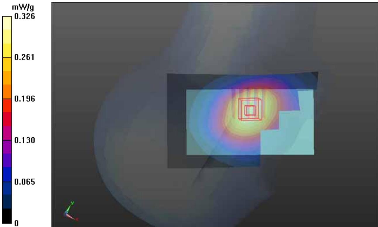
**P570 LTE 5\_QPSK\_10M\_Right Tilted\_Ch20600\_1RB\_Offset 0****DUT: 120626C35**
