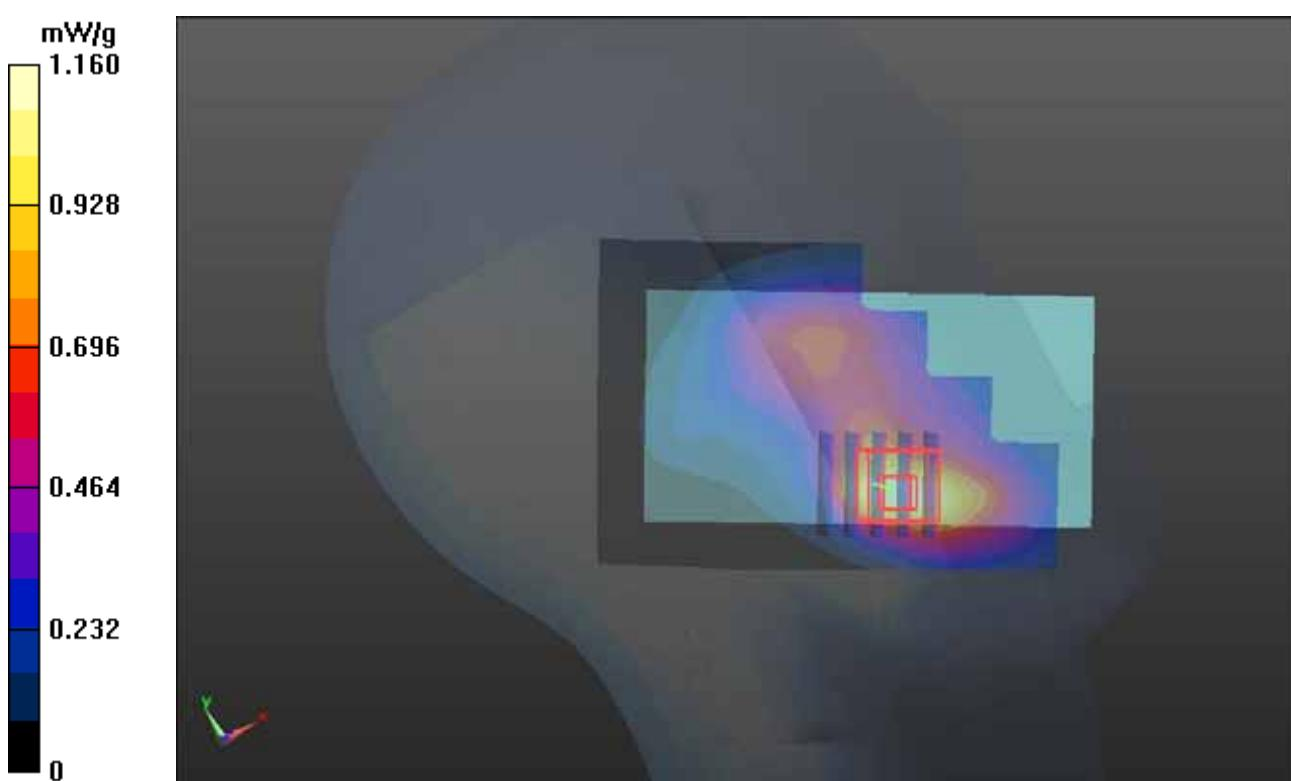
**P550 LTE 17\_QPSK\_10M\_Right Cheek\_Ch23790\_25RB\_Offset 12****DUT: 120626C35**
