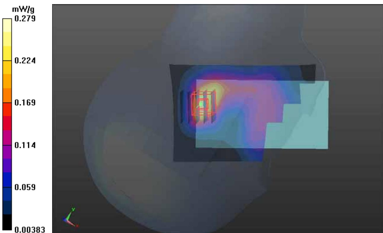
**P582 LTE 4\_QPSK\_10M\_Left Cheek\_Ch20350\_25RB\_Offset 12****DUT: 120626C35**
