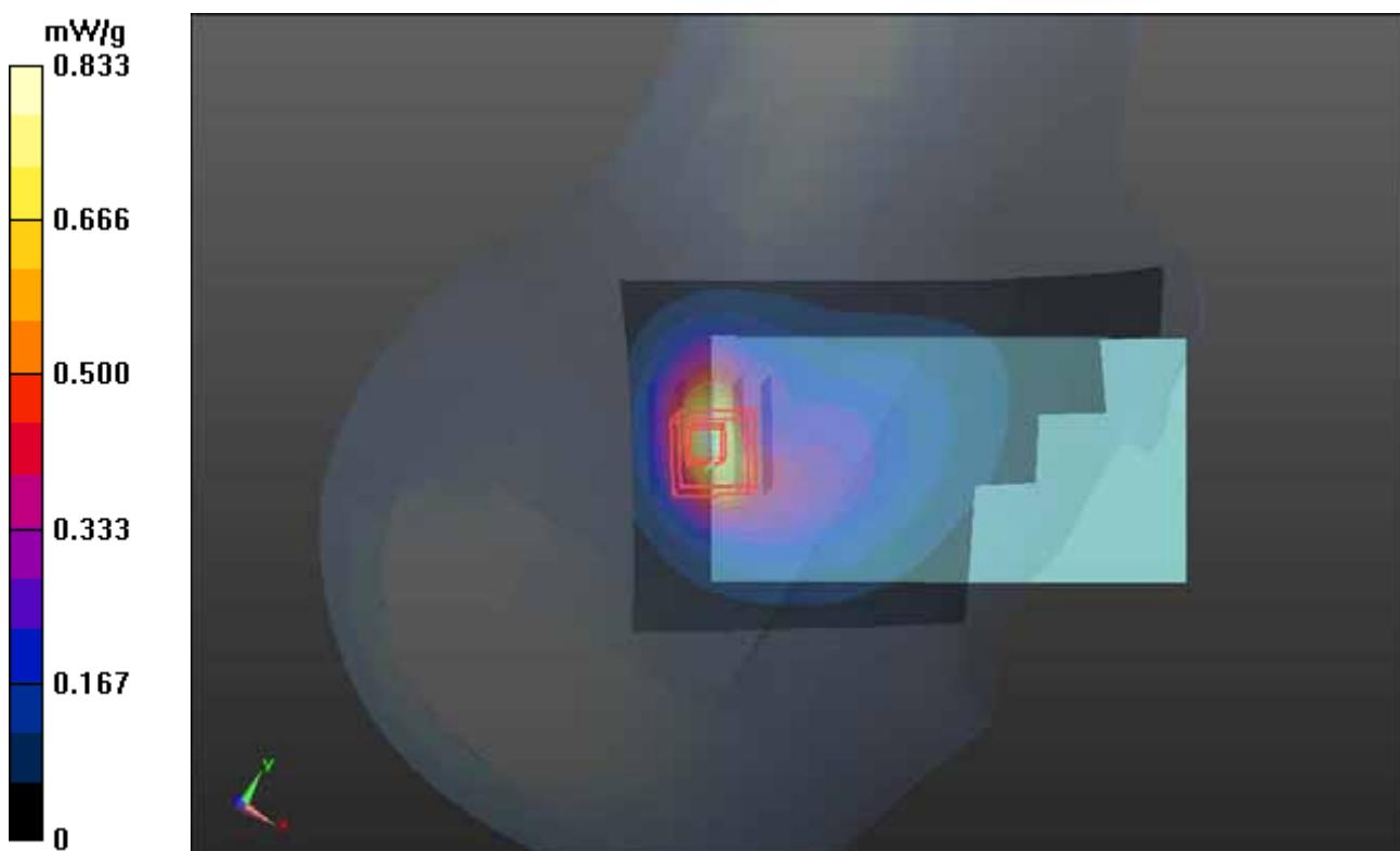
**P560 LTE 17\_QPSK\_10M\_Left Cheek\_Ch23790\_1RB\_Offset 49****DUT: 120626C35**
