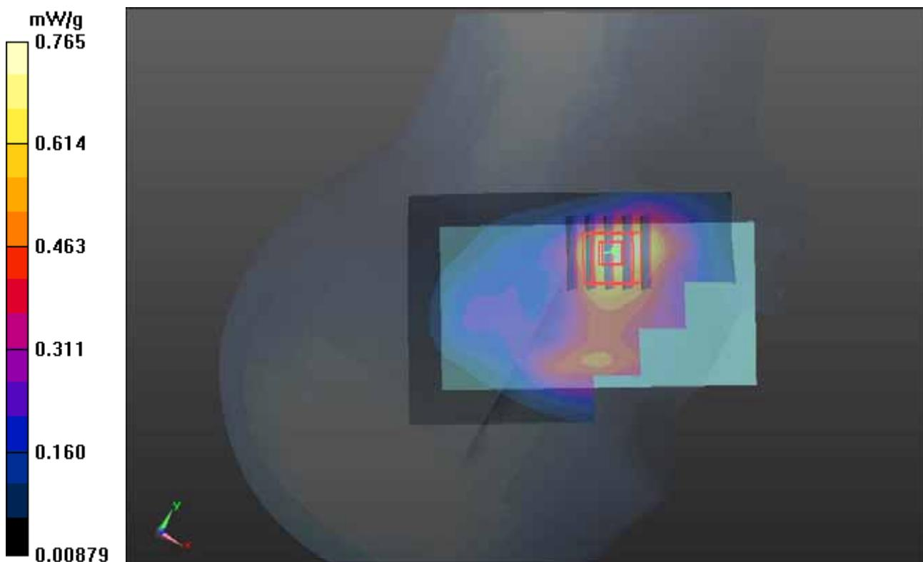
**P06 GSM1900\_GPRS10\_Right Tilted\_Ch810****DUT: 120626C35**
