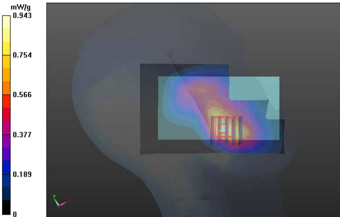
**P594 LTE 4\_16QAM\_10M\_Left Cheek\_Ch20350\_1RB\_Offset 49****DUT: 120626C35**
