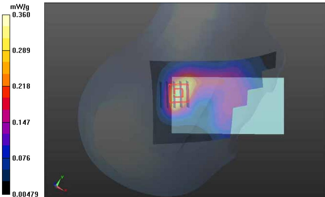
**P586 LTE 4\_QPSK\_10M\_Left Cheek\_Ch20350\_1RB\_Offset 0****DUT: 120626C35**
