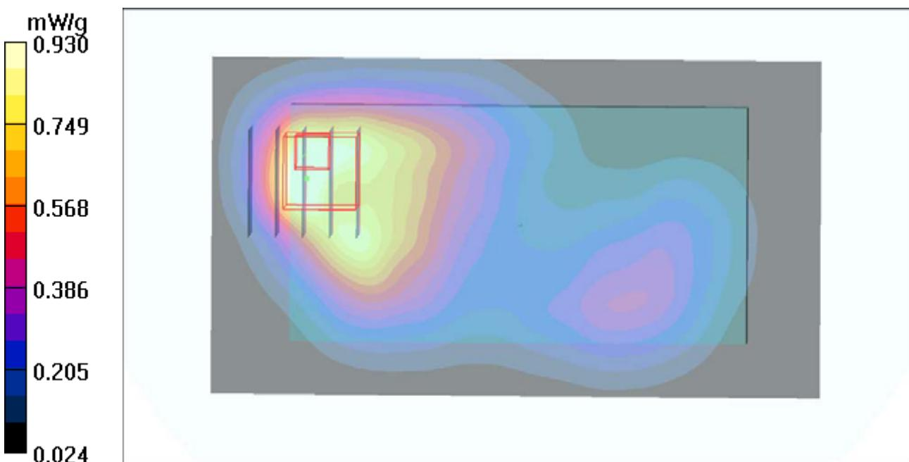
**P85 GSM1900\_GPRS10\_Rear Face\_1cm\_Ch512****DUT: 126026C35**
