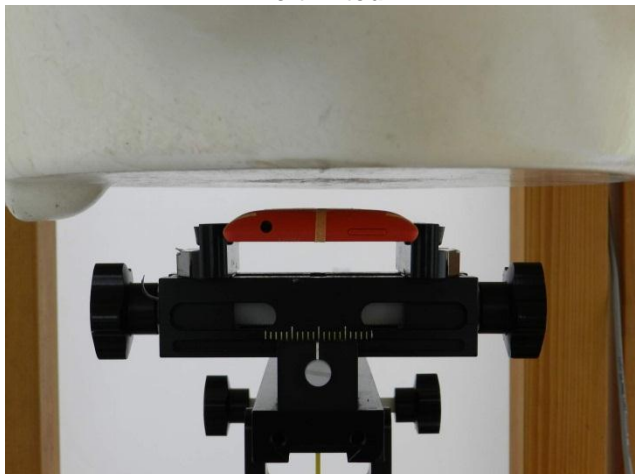
Back of the DUT with Phantom 1 cm Gap (without Headset)
