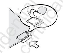
3. Insert the SIM card tray into its slot.
