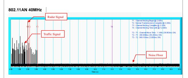
**NOTE:** T1 denotes the start of Channel Move Time upon the end of the last Radar burst. T2 denotes the data transmission time of 200ms from T1. T3 denotes the end of Channel Move Time.T4 denotes the 10 second from T1 to observe the aggregate duration of transmissions.
