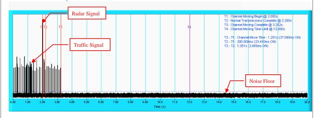
**NOTE:** T1 denotes the start of Channel Move Time upon the end of the last Radar burst. T2 denotes the data transmission time of 200ms from T1. T3 denotes the end of Channel Move Time.T4 denotes the 10 second from T1 to observe the aggregate duration of transmissions.
