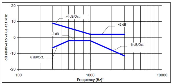
Figure 8.4a Magnetic field frequency response for WDs with a field ≤ −15 dB (A/m) at 1 kHz
