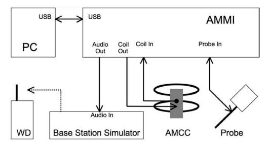
Figure 5.1: T-Coil setup cabling
