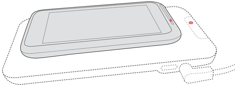
As the battery is being charged, the notification LED shows a solid orange light. The light turns to solid green when the battery is fully charged.
