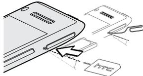
2. Pull the SIM card tray out, and place the SIM card (contacts facing down) into the tray.
