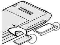
3. Insert the SIM card tray into its slot.
