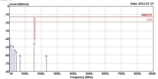
Site : 966 Chamber 5 Condition : PART27 3m EIRP\_RSE\_1G~19G\_3 VERTICAL
