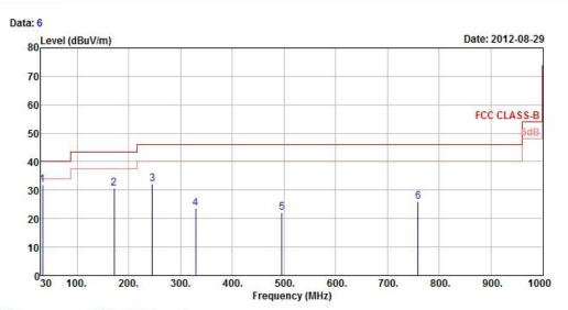
Site : 966 Chamber 5 Condition : FCC CLASS-B 3m ANT\_30M~1G\_LF VERTICAL
