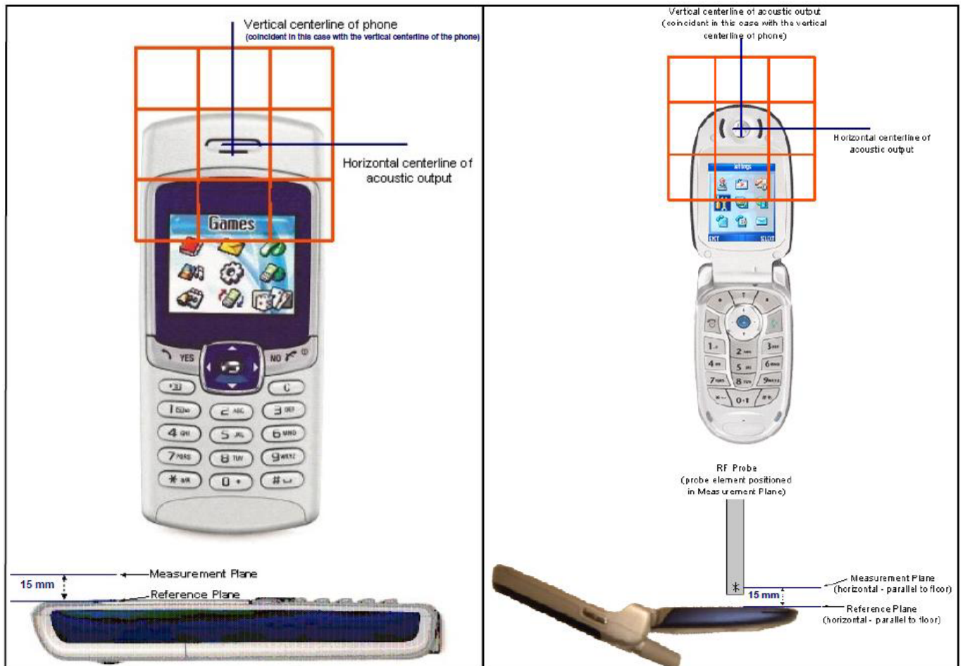
Fig-3.5 EUT Reference and Plane
