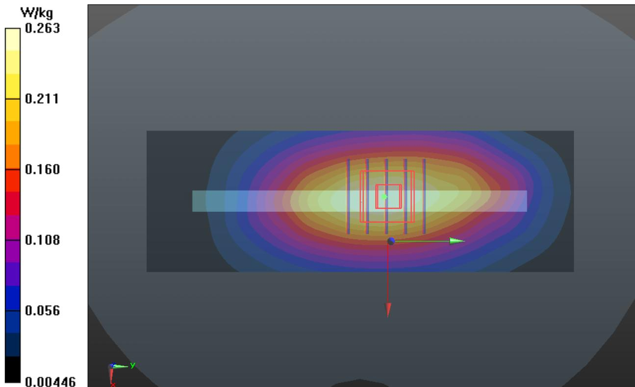
**P338 LTE 13\_16QAM\_10M\_Left Side\_1cm\_Ch23230\_1RB\_Offset 49**
