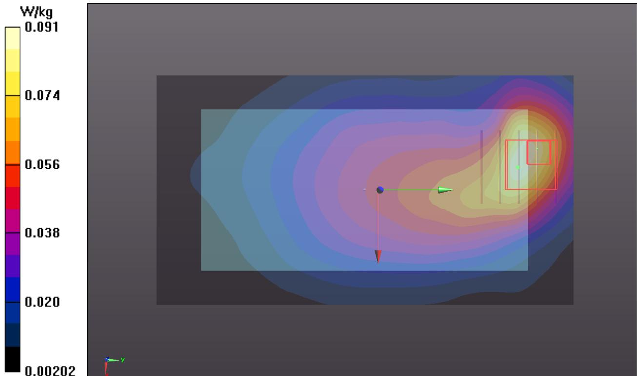
**P239 LTE 13\_QPSK\_10M\_Rear Face\_1cm\_Ch23230\_1 RB\_Offset 0\_Earphone**
