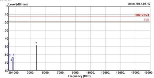
Site : 966 Chamber 5 Condition : PART22/24 3m EIRP\_RSE\_1G~19G\_3 HORIZONTAL
