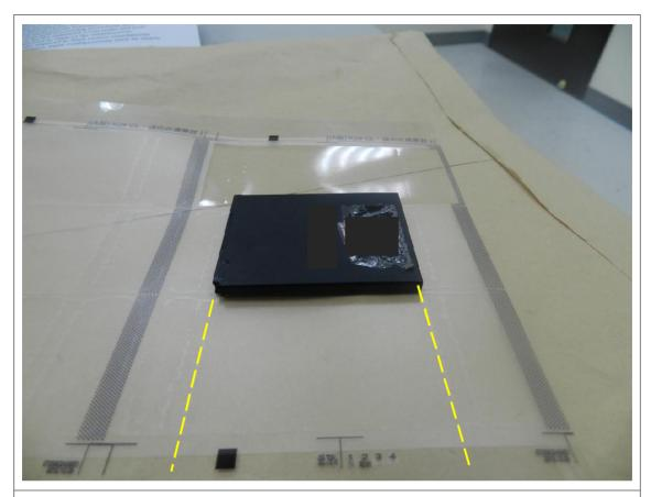
1. Place the battery on the film and align the battery to the lines.
