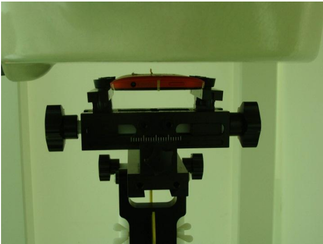
Back of the DUT with Phantom 1 cm Gap (DUT without Headset)
