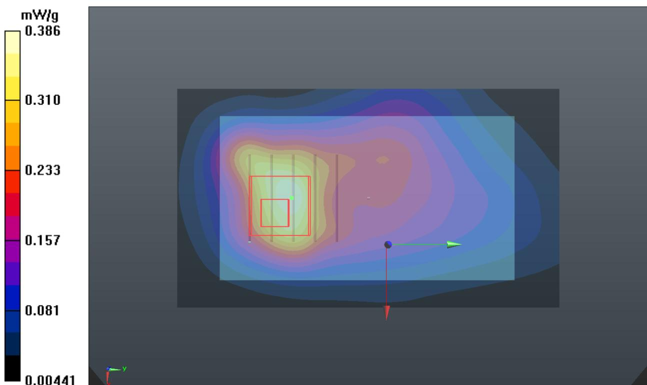
**P61 CDMA2000 BC15\_RC3+SO32\_Rear Face \_1cm\_Ch425\_Battery2\_Earphone****DUT: 120508C07**
