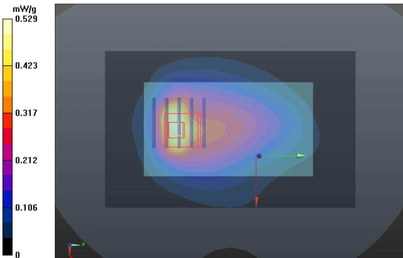
**P41 CDMA2000 BC0\_RC3+SO32\_Rear Face\_1cm\_Ch1013\_Battery2\_Earphone****DUT: 120508C07**
