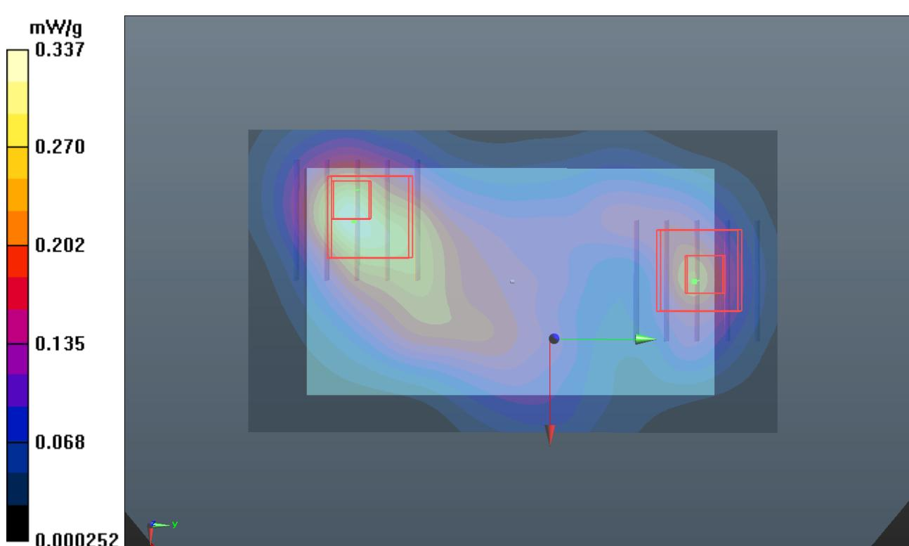
**P60 CDMA2000 BC15\_RC3+SO32\_Rear Face \_1cm\_Ch425\_Battery1\_Earphone****DUT: 120508C07**
