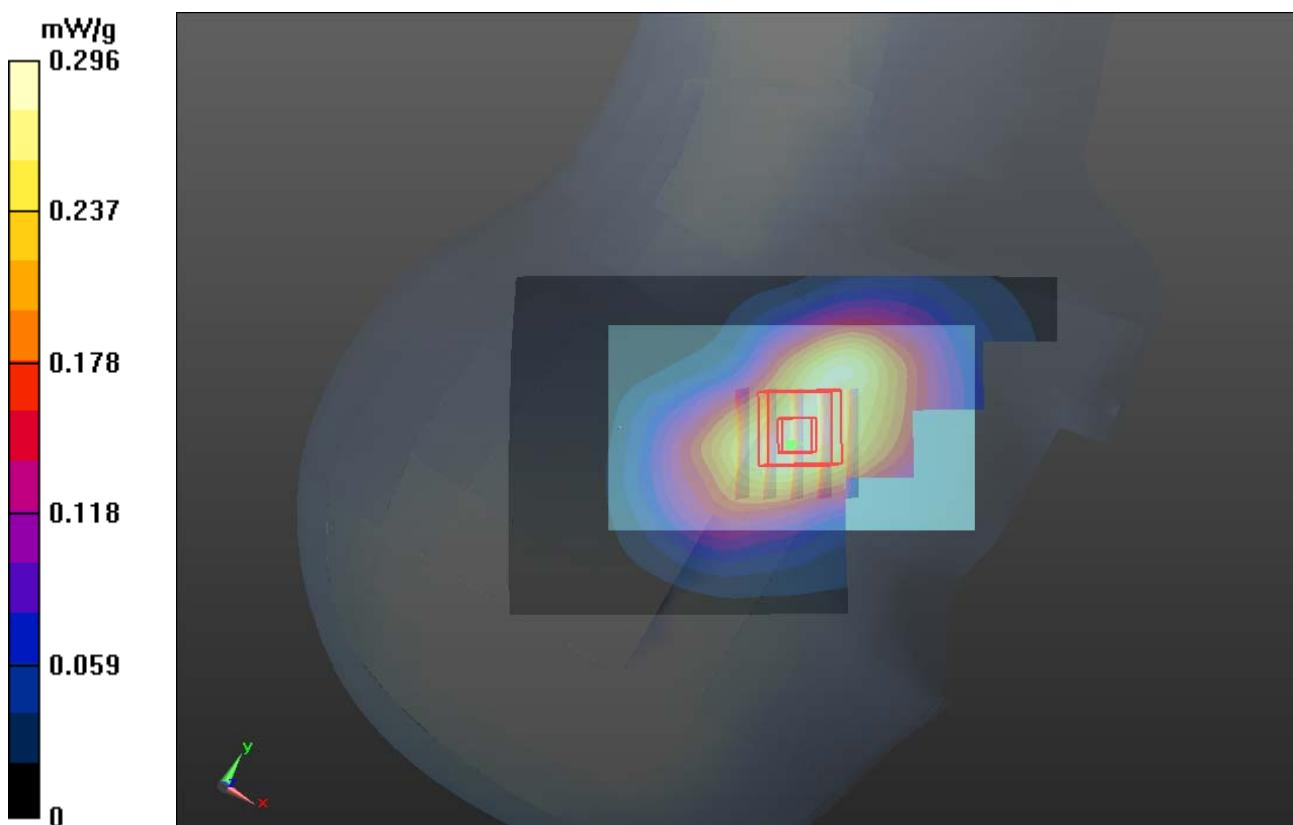
**P02 CDMA2000 BC0\_RC3+SO55\_Right Tilted\_Ch1013\_Battery1****DUT: 120508C07**
