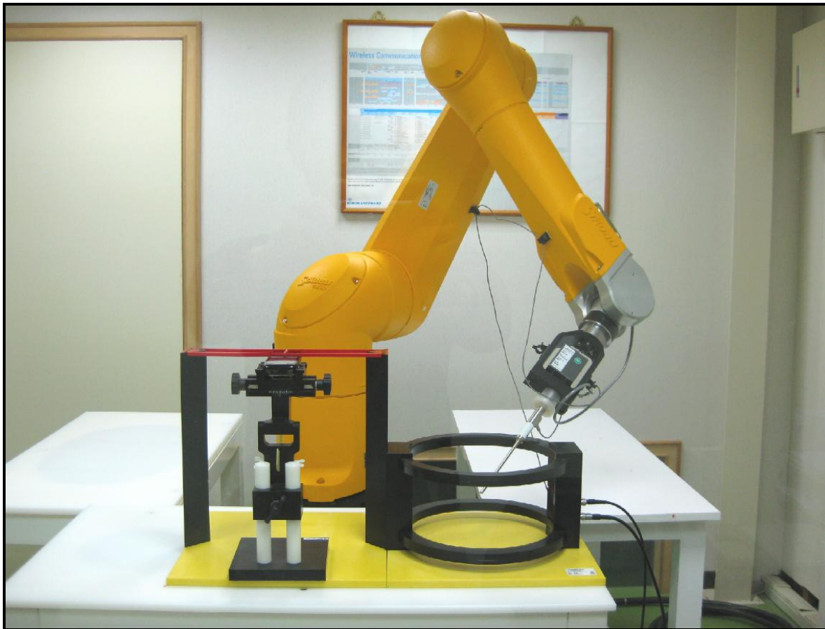
Figure 4.2: T-Coil setup with HAC Test Arch and AMCC
