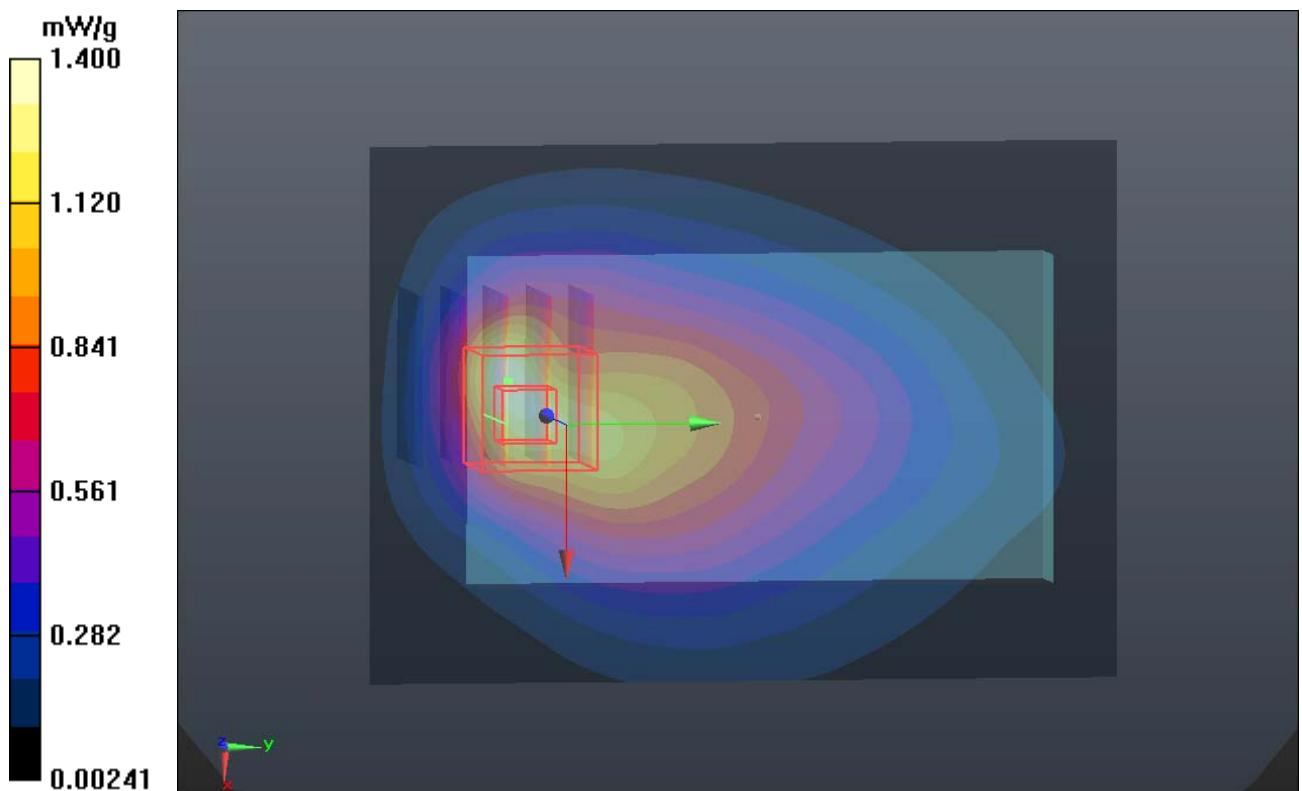
**P107 GSM850\_GPRS10\_Rear Face\_Ch251\_Battery1\_Earphone1****DUT: 120405C02**
