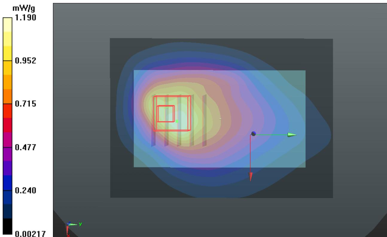
**P109 GSM850\_GPRS10\_Rear Face\_Ch189\_Battery2\_Earphone2****DUT: 120405C02**
