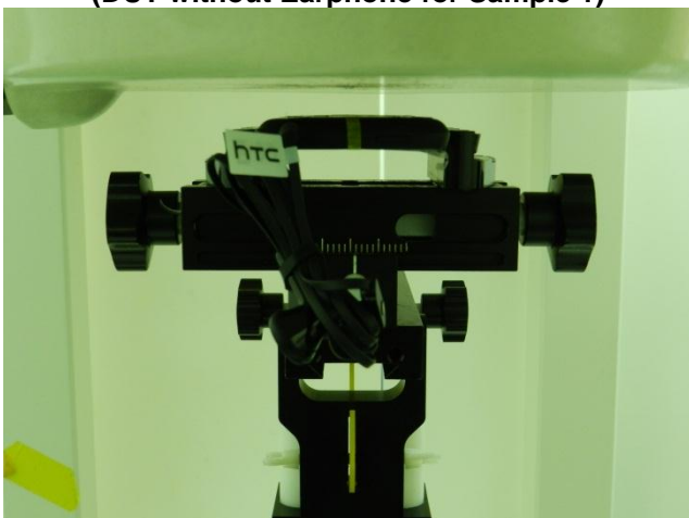
Back of the DUT with Phantom 1 cm Gap (DUT with Earphone for Sample 1)
