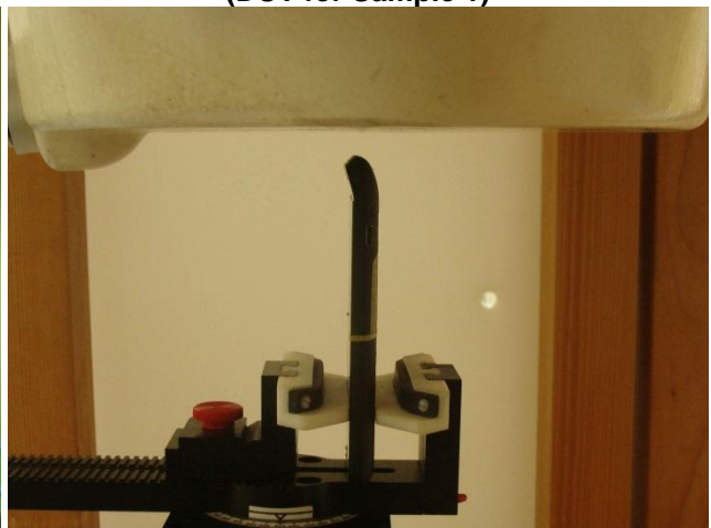
Bottom Side of the DUT with Phantom 1 cm Gap (DUT for Sample 2)
