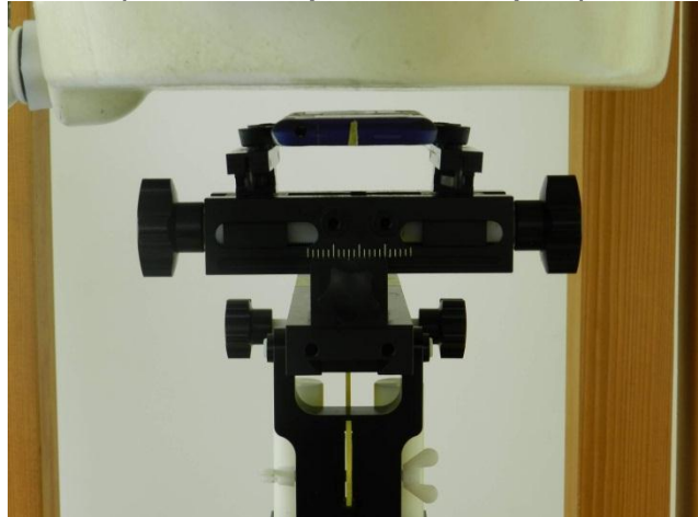
Back of the DUT with Phantom 1 cm Gap (DUT without Earphone for Sample 2)
