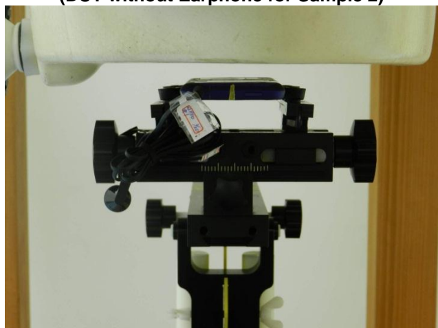
Back of the DUT with Phantom 1 cm Gap (DUT with Earphone for Sample 2)
