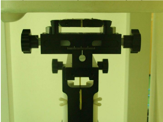
Back of the DUT with Phantom 1 cm Gap (DUT without Earphone for Sample 1)
