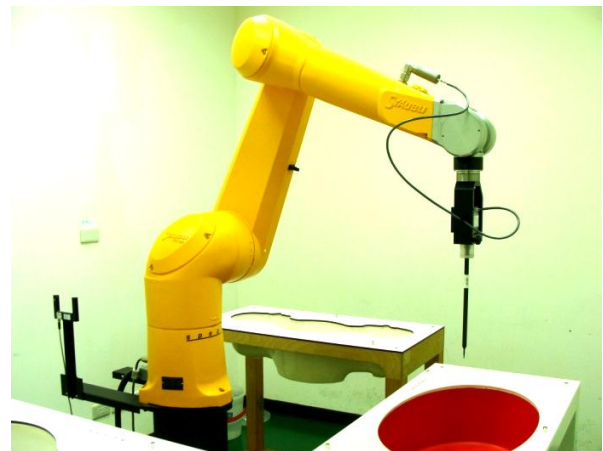
Fig 5.8 Photo of DASY5
