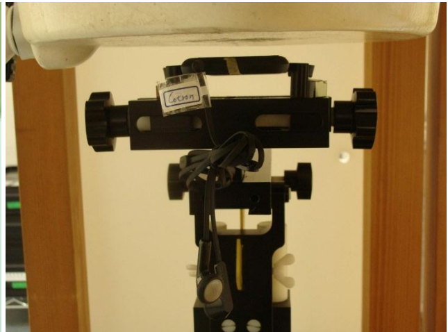
Back of the DUT with Phantom 1 cm Gap (DUT with Earphone 2)
