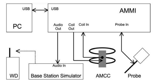
Figure 5.1: T-Coil setup cabling
