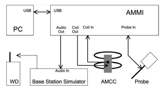
Figure 5.1: T-Coil setup cabling
