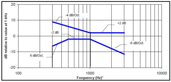
Figure 8.4a Magnetic field frequency response for WDs with a field ≤ −15 dB (A/m) at 1 kHz
