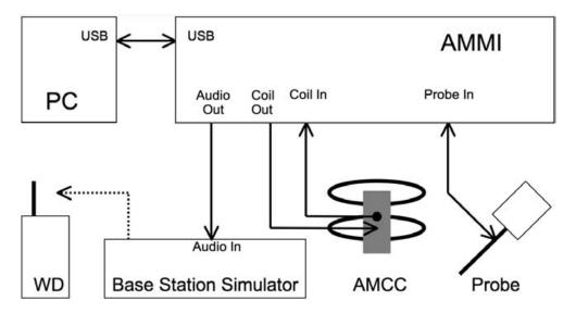
Figure 5.1: T-Coil setup cabling
