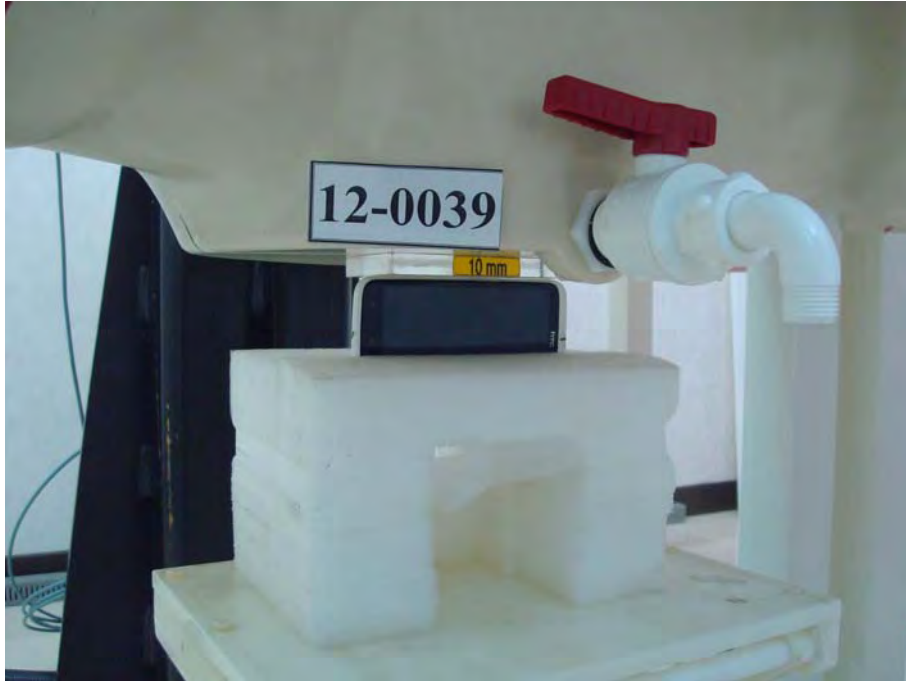
Figure 11. Body SAR Test Setup (Flat Section)
