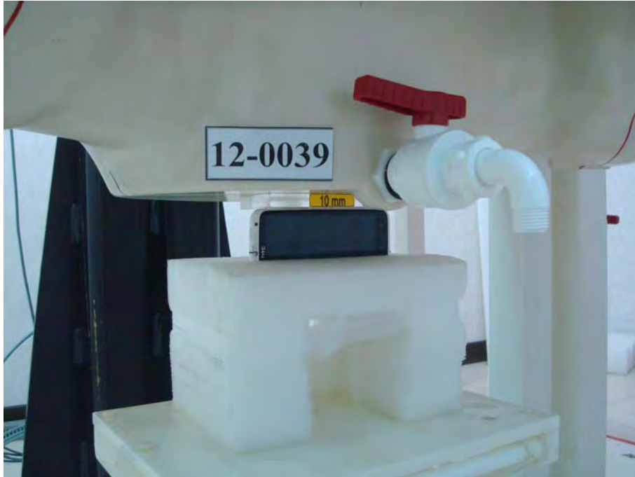
Figure 10. Body SAR Test Setup (Flat Section)
