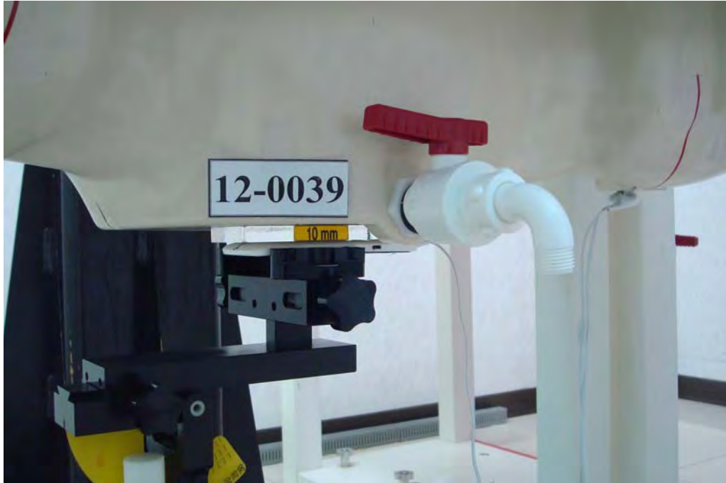
Figure 6. Body SAR Test Setup (Flat Section)
