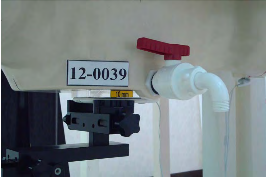
Figure 8. Body SAR Test Setup (Flat Section)
