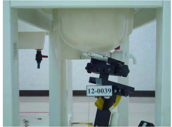
Figure 2. Right Head SAR Test Setup (Tilted)
