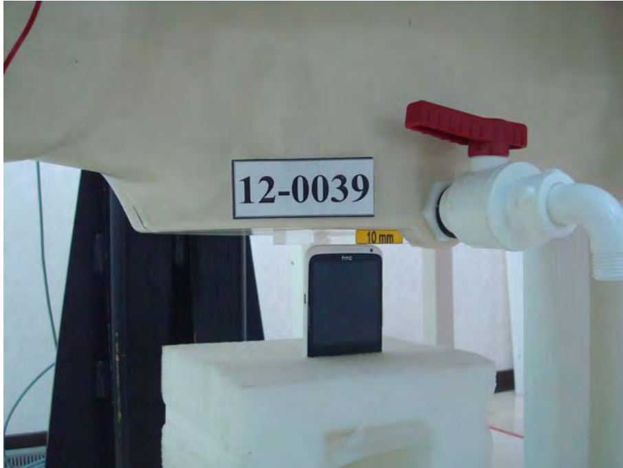
Figure 12. Body SAR Test Setup (Flat Section)
