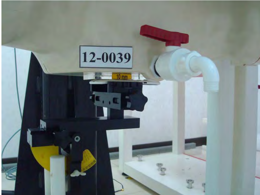
Figure 5. Body SAR Test Setup (Flat Section)
