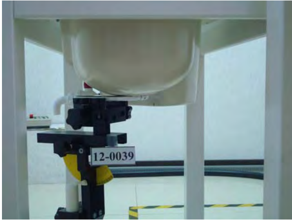
Figure 3. Left Head SAR Test Setup (Cheek)
