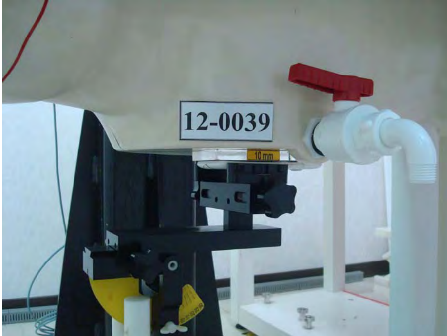
Figure 7. Body SAR Test Setup (Flat Section)
