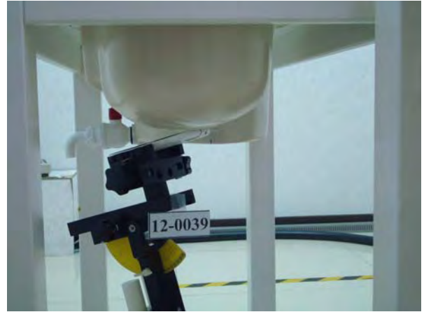
Figure 4. Left Head SAR Test Setup (Tilted)
