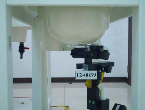
Figure 1. Right Head SAR Test Setup (Cheek)
