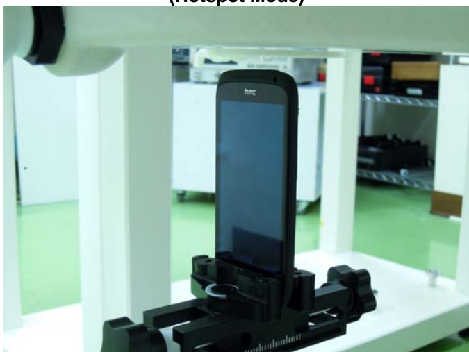
Top Side of DUT with 1 cm Gap (Hotspot Mode)
