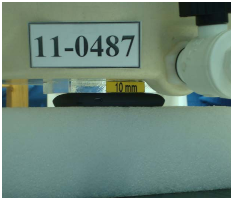
Figure 6. Body SAR Test Setup (Flat Section)
