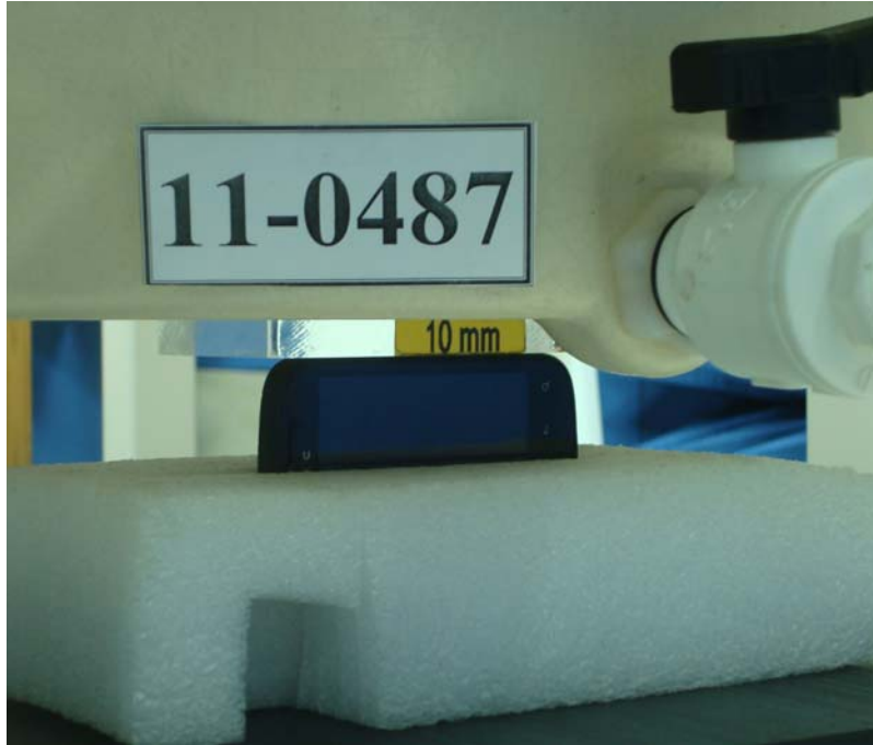
Figure 8. Body SAR Test Setup (Flat Section)
