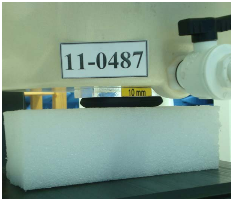
Figure 5. Body SAR Test Setup (Flat Section)
