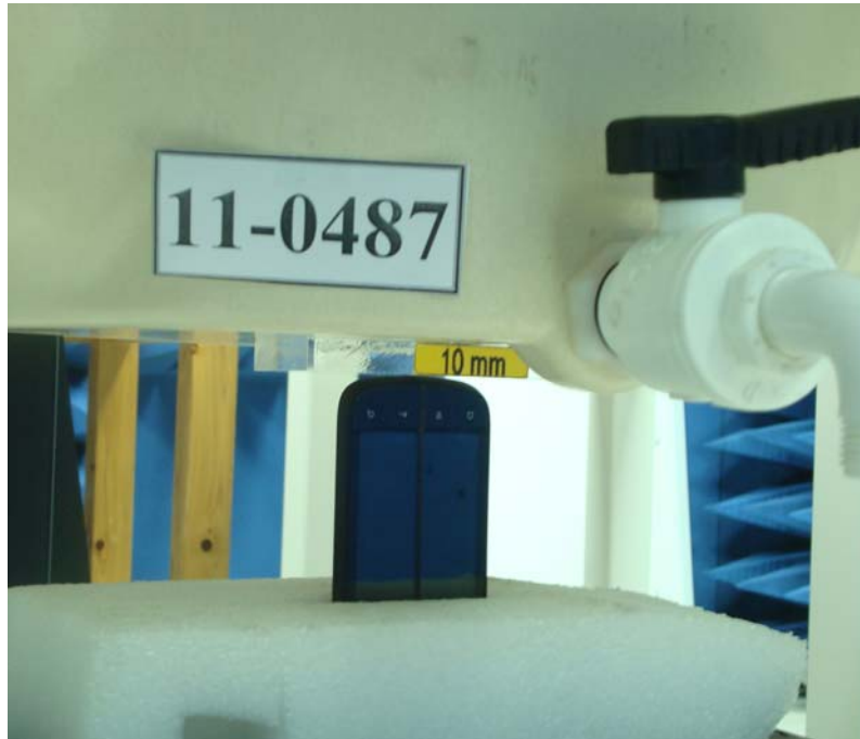
Figure 9. Body SAR Test Setup (Flat Section)
